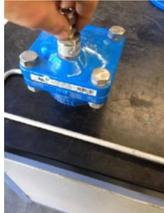
2. Screw in male connector by hand until firm (Use a sealant or thread tape to seal).
