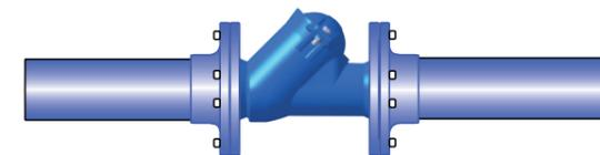
A horizontal installation requires a minimum flow velocity of 1 - 1.5 m/s to open effectively. A recommended back pressure of 0.6 bar is needed when closing the valve.
