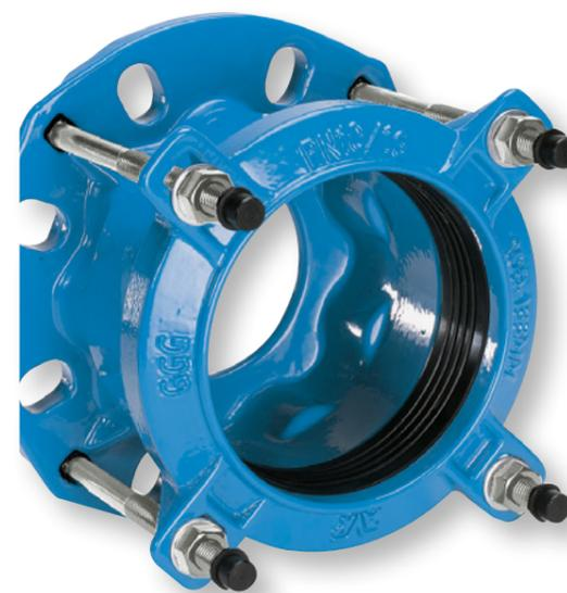
The AVK Supa® universal straight couplings, step couplings and flange adaptors are suitable for uPVC, Cast Iron, Ductile Iron, Steel and AC pipes. The couplings range from DN40-400 and are suitable for water and wastewater applications.
