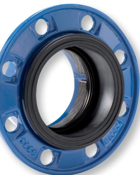
AVK's combi-flange system comprises tensile combi-flanges for PE, PVC and Ductile Iron pipes in DN50-300 as well as non-tensile combi-flanges for PVC, Ductile Iron and Steel pipes in DN50-600. The combi-flanges are suitable for water and wastewater applications.
