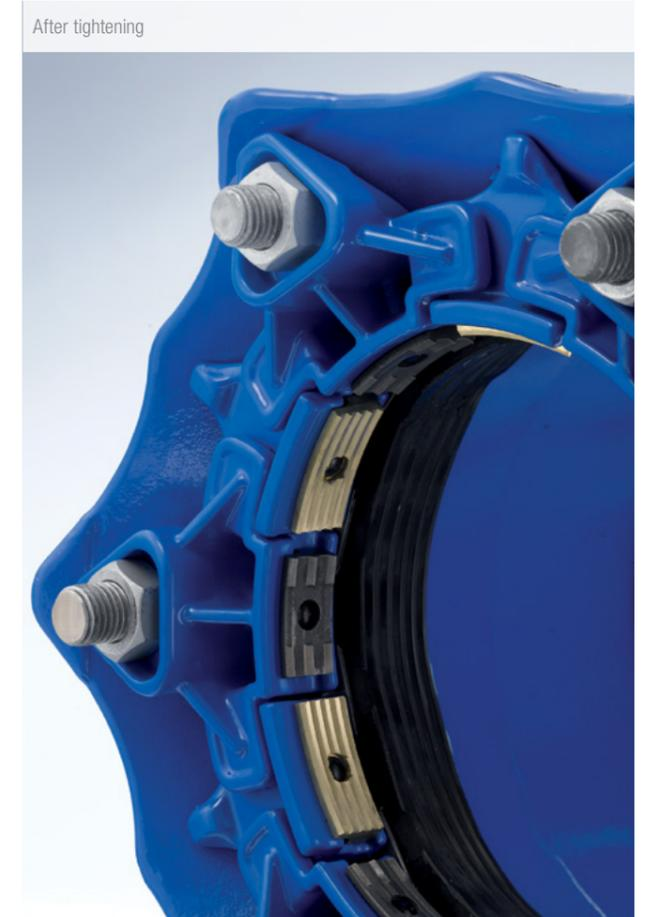
The patented SupaGrip™ sealing support system features a flexible bracket, and combined with the unique grip design, SupaGrip™ provides superior tightness and tensile resistance on all pipe dimensions and materials.
