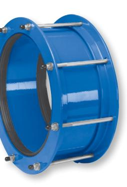
AVK's range of fabricated fittings comprises non-tensile straight couplings, step couplings and flange adaptors in DN350-2000. The range is suitable for Ductile and grey Cast Iron, Steel, uPVC and GRP pipes for water and wastewater applications up to 25 bar.
