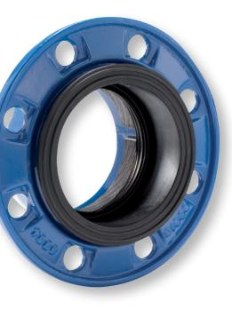
AVK's combi-flange system comprises tensile combiflanges for PE, PVC and Ductile Iron pipes in DN50-300 as well as non-tensile combi-flanges for PVC, Ductile Iron and Steel pipes in DN50-600. The combi-flanges are suitable for water and wastewater applications.
