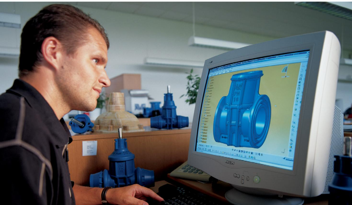
Computer simulation using 3-D software simulates strength and pressure load on all parts of the product, enabling us to reinforce and optimise possible weak zones at the very early stages of development.
