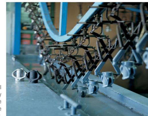
During vulcanisation, the metal wedge core remains untouched by outside bodies which may impede the bonding process between the metal core and the rubber.
