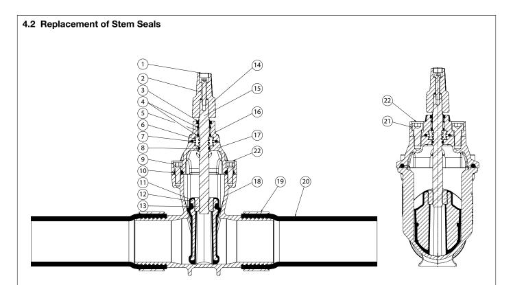
This can be carried out with valve under pressure in the pipeline, but take care over step 'a' to ensure a seal is formed between wedge and bonnet.
