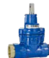
Series 03/85 Service connection valve with tensile screw coupling for PE pipes / external thread DN25-32 PN16 Ductile iron
